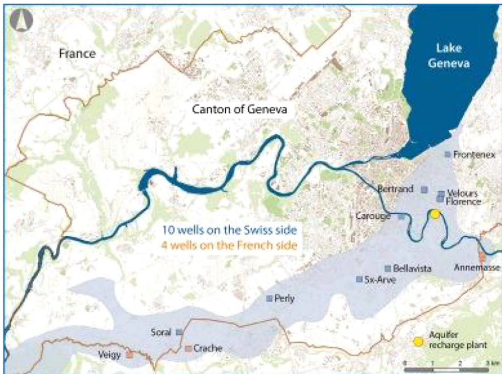
Fig. 2. Location of the wells (drinking water supply) in the Genevese aquifer (water flow directions are from river Arve to the lake and to the west part of the canton).
